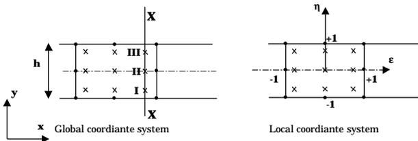
**Figure 1 - An 8-noded quadrilateral element forming part of a beam**
