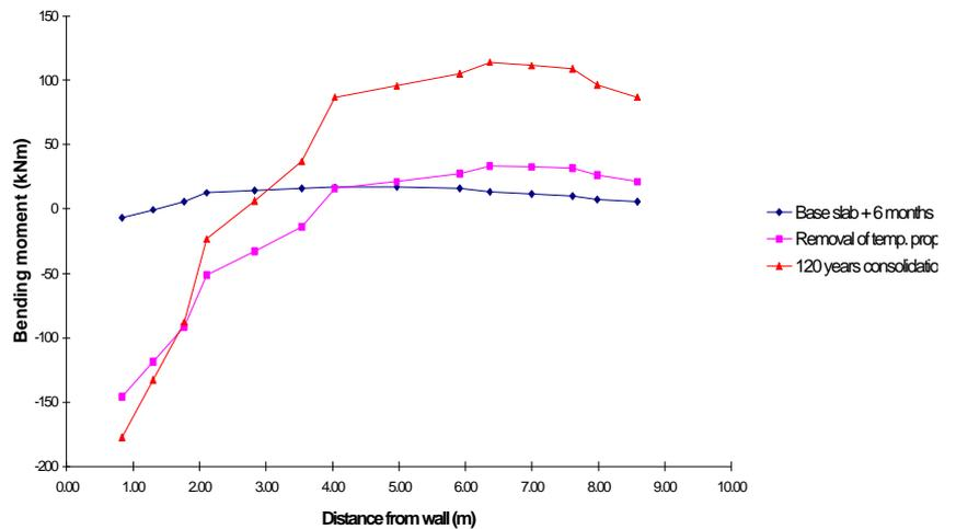
Bending moment profiles within the permanent prop slab at three different stages of the analysis were calculated from horizontal stresses at integration points across the width of the slab. The distribution of integration points within an LST element makes it difficult to calculate bending moment from element stresses, and so the profile stops just short of the triangle.
